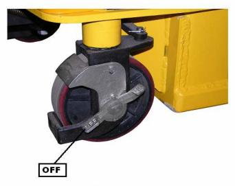
To activate the parking brake, press down on the brake pedal
