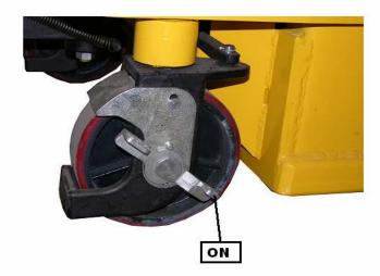
To release the pariking brake, press down on the brake pedal
